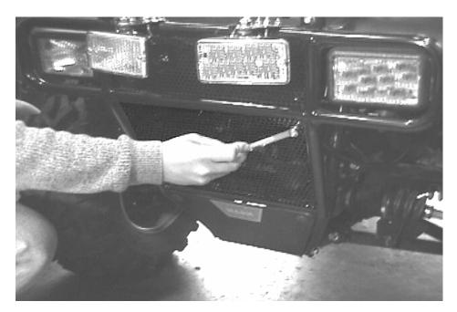
2. Place the mounting plate into position with the bent handle on the top of the mounting plate and the opening for the fairlead towards the bottom. Attach the top two mounting plate holes with two of the bolts that where removed in step one.
