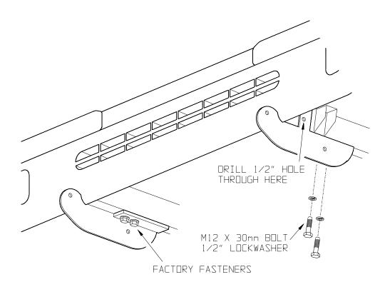
5. Install the side members onto the outsides of the frame extensions as shown in Figure 3.
