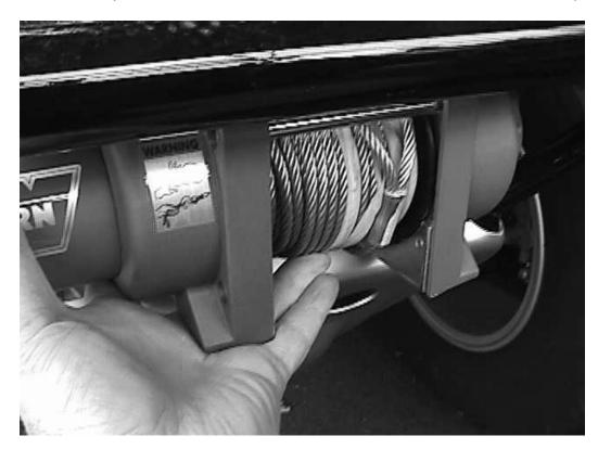
**STEP 3:** While holding the winch up out of the way, slip the mounting plate into position under the winch. Do not bolt down the winch at this time.
