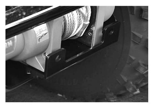
**STEP 4:** Place the ¼-20 u-bolts into position around the frame and bumper tubes and into the mounting bracket. Tighten with the ¼-20 hex nuts and lock washers.
