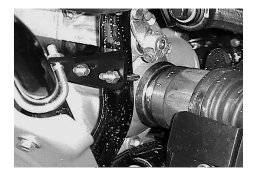
**STEP 5:** Attach the cast hawse fairlead that came with the winch onto the front two tabs on the mounting plate. The hawse fairlead will have to be removed from the fairlead plate that came with the winch, use the same hardware to attach it to the mounting plate.
