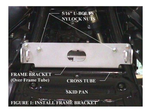
Install both U-Bolts over the top of the frame tubes and into the frame bracket (Fig. 2). The 5/16" U-Bolts should be just in front of the vertical frame tubes forward of the motor as shown.
