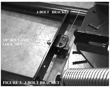
Run the winch cable over the roller fairlead and down to the J-bolt bracket. Using a 1/4" dia J-bolt, hook the loop on the end of the winch cable and slide the threaded end of the J-bolt into the slotted hole in the J-bracket. Terminate the end of the J-bolt with a 1/4"dia nylock nut. Tighten the nut until the winch cable is snug inside the J-bolt as shown in figure 4.
