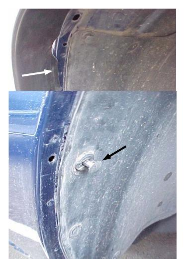
If it is necessary to remove any of the plastic rivets securing the fender liner, carefully lift and remove the inner rivet pin, then the rivet.
