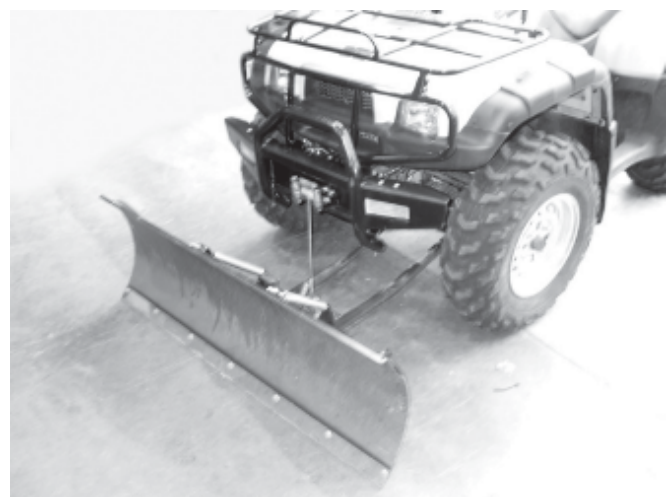
Figure 5 Completed Winch and Plow Assembly
