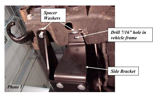
2. Using hole in the Side Brackets as a guide, mark the vehicle frame for drilling. Remove the brackets and drill a 7/16" hole at each marked location.
