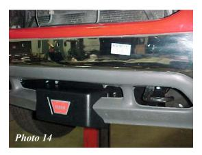
12. Install the bumper and tighten securely. Be sure to reattach fog light sockets. Reinstall grille.
