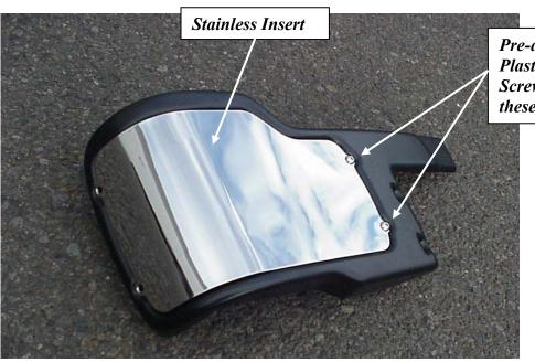
Pre-assemble Inserts to the Plastic Panels using the Screws and Locknuts at these positions only.
