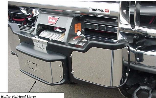
To install, be sure the metal tab on the back side is engaged behind one roller, then snap other end into place. To remove, pull sharply at one end. The cover is intentionally a tight fit to assure that it stays in place.
