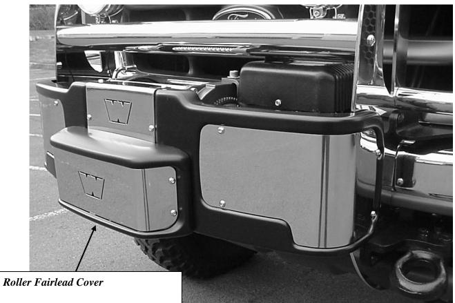
To install, be sure the metal tab on the back side is engaged behind one roller, then snap the other end into place. To remove, pull sharply at one end. The cover is intentionally a tight fit to assure that it stays in place.
