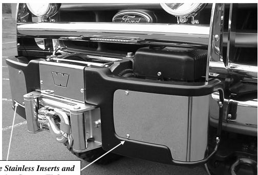
Install the Stainless Inserts and the remaining Screws. Tighten all the screws securely.
