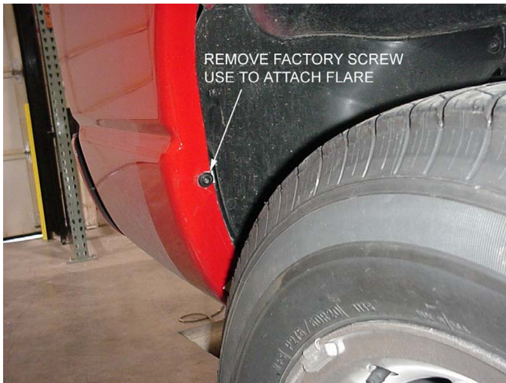
Figure 1 Rear factory screw, right side fender
