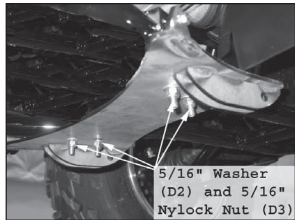
Figure 6 Completed Plow Mount
