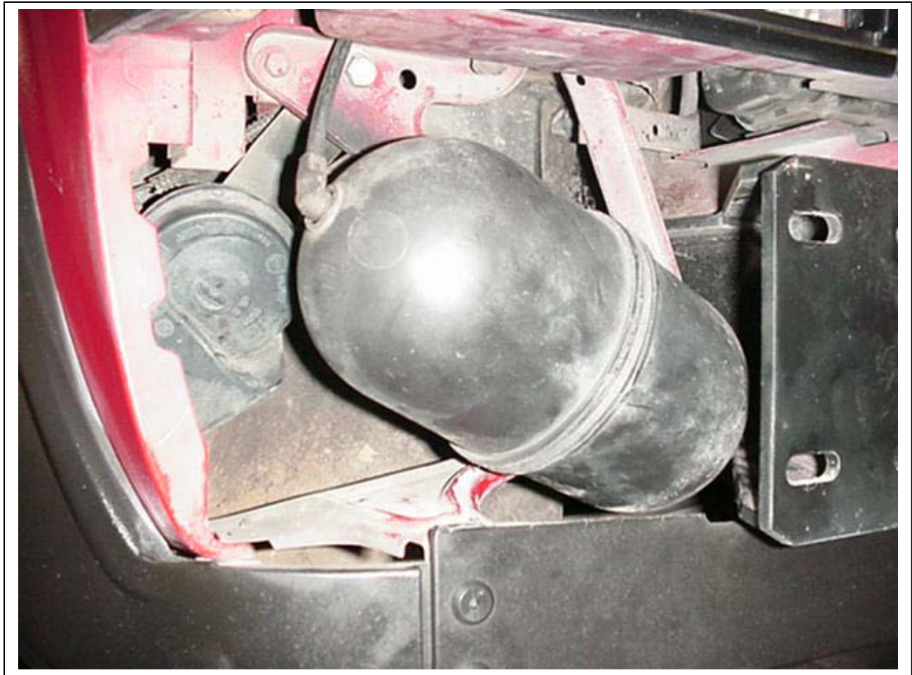
Figure 6 A, Vacuum canister, final assembly. Attach canister to lower strap and hold it in place to mark the upper hole. Remove canister and drill \frac{1}{4} " hole in fender support and re-attach canister.
