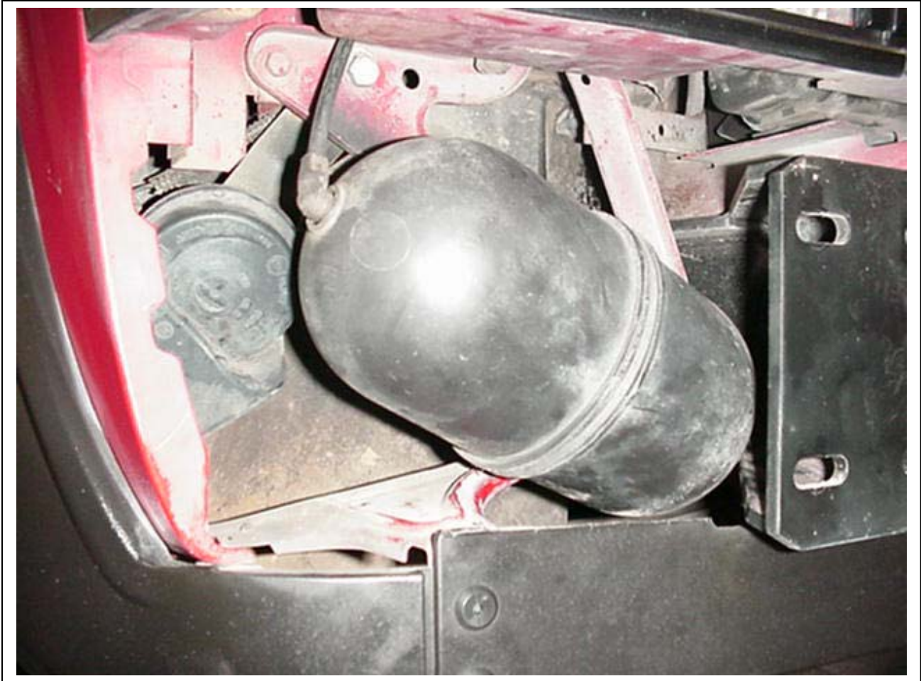
Figure 6 A, Vacuum canister, final assembly. Attach canister to lower strap and hold it in place to mark the upper hole. Remove canister and drill ¼" hole in fender support and re-attach canister.
