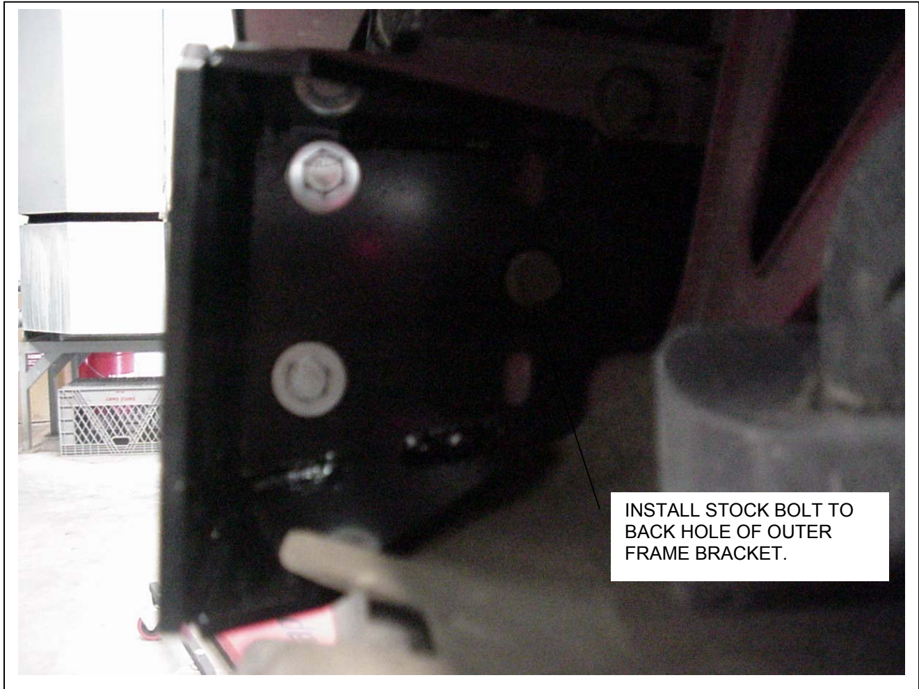
Figure 4, Driver's side view of out frame bracket.
