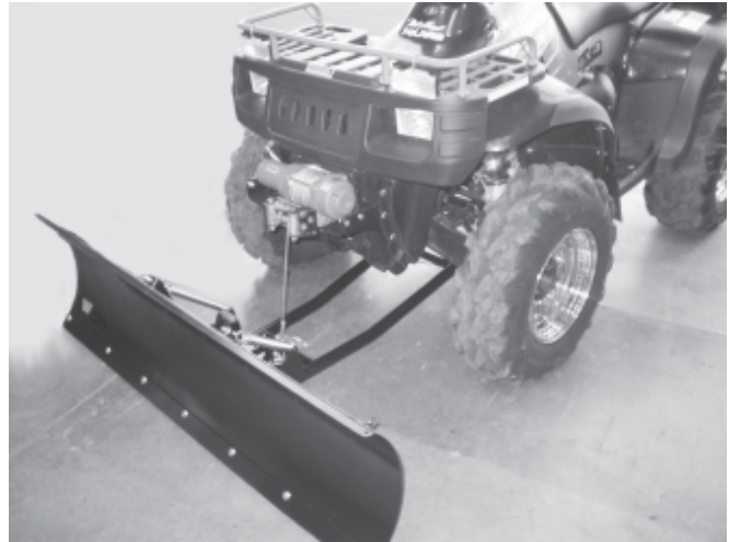
Figure 7 Completed Winch and Plow Assembly
