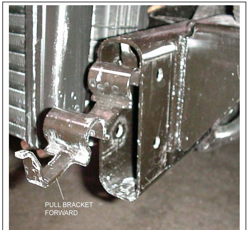
Figure 5 Left frame tube “anti-crush” brackets pried up for access inside the frame tube
