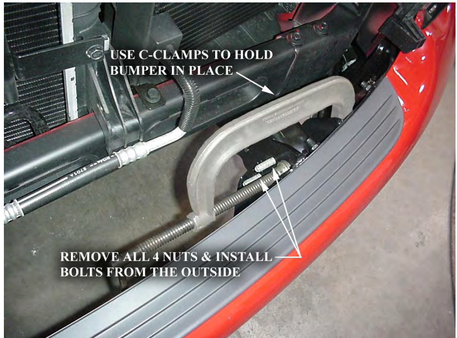
Figure 7: Remove bumper/frame bolts
