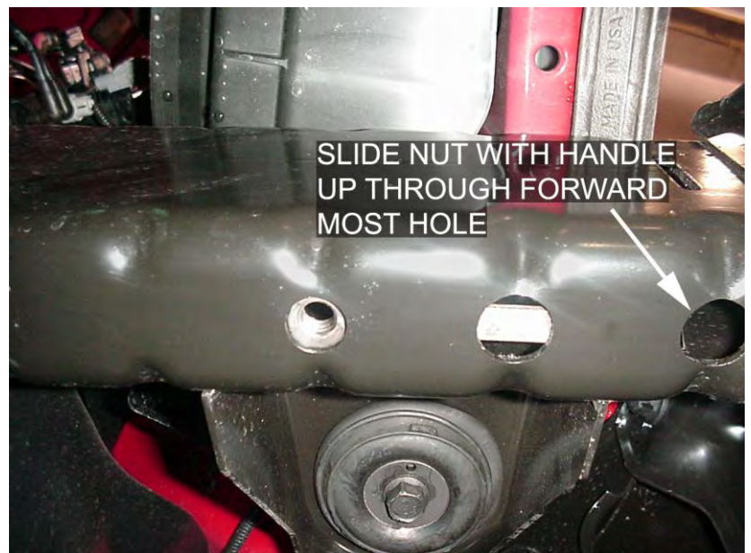
Figure 10: Location of Nut with Handle (left frame rail viewed from bottom).
