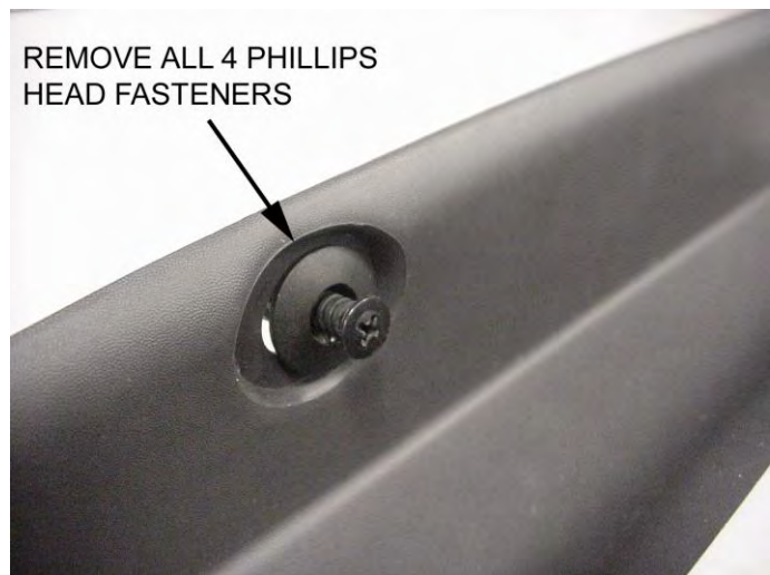
Figure 6: Remove gray plastic fascia from the bumper.
