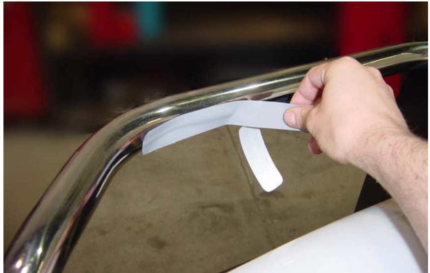
Figure 8: Stick to centerline first to minimize air bubbles.
