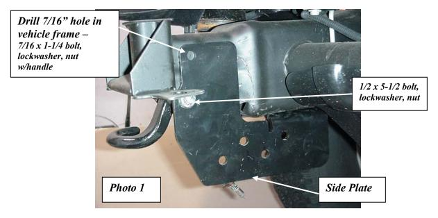
3. Refer to **Photo 2** and push the Side Plate up tight against the bottom of the frame. Using the hole in the plate as a guide, drill a 7/16" hole up into the bottom of the frame. Secure with the bolt indicated and a nut with wire handle. Tighten this lower bolt and the tow hook bolts securely.
