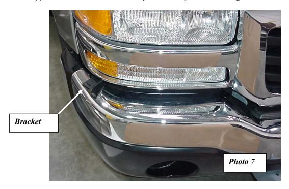
7. Align the slot in the bracket with the hole in the bottom of the Brush Guard. Install the 1/4" self-tapping bolt from the bottom up and tighten securely. **Photo 8**. Tighten the 3/8" bolt at the Bracket to bumper connection.
