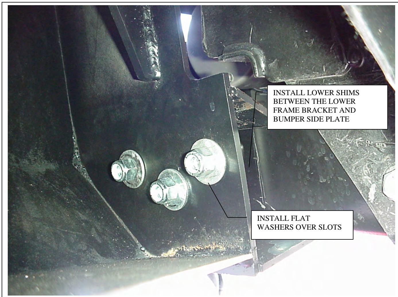
Figure 5, Bumper, Shims, Carriage Bolts, Flat Washers, Lock Nuts
