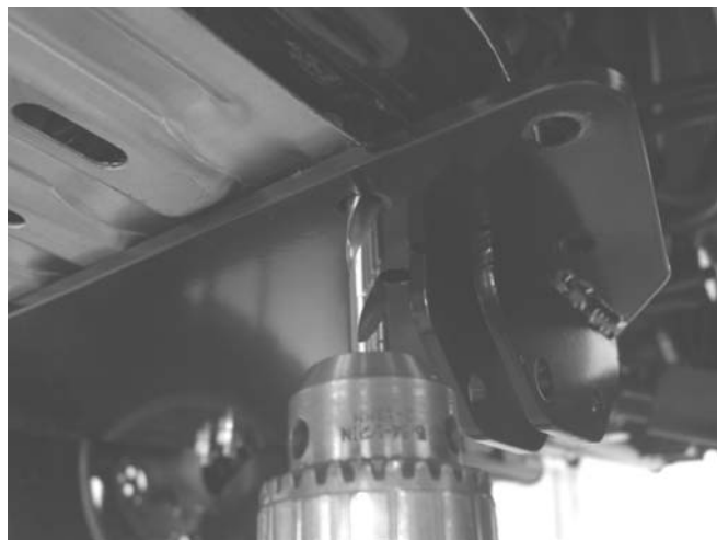
Figure 3 Drill Rear Holes
