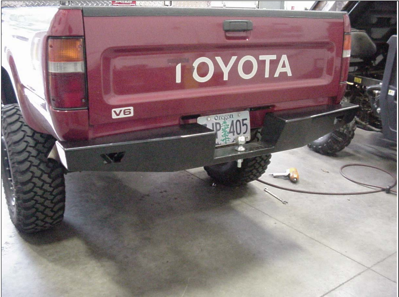
Figure 5, Bumper aligned and mounting hardware torqued.
