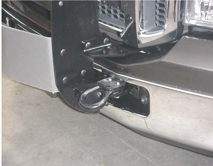
Figure 8 - Exploded view of LH tow loop/Frame Extension
