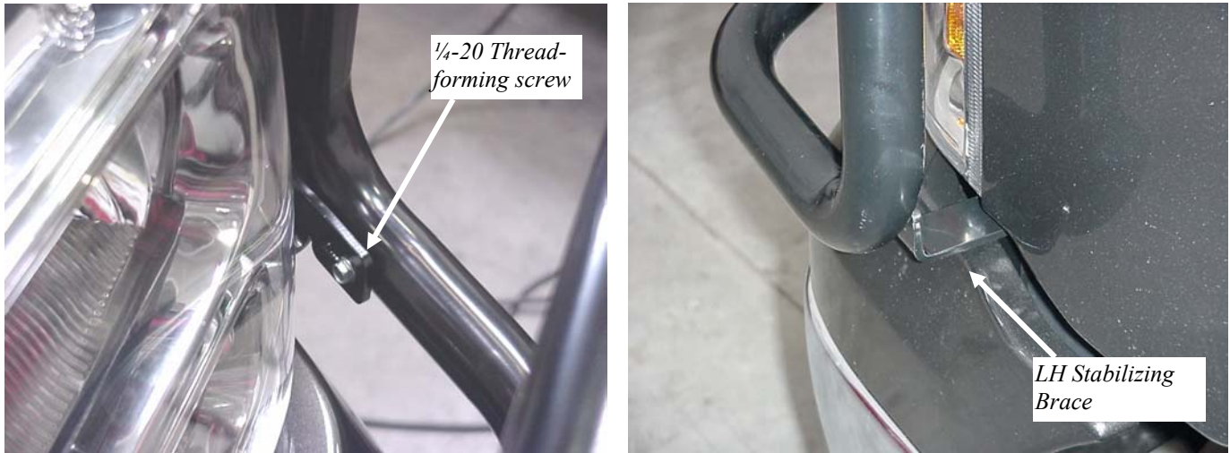
Figure 4-5 Stabilizing Brace detail
