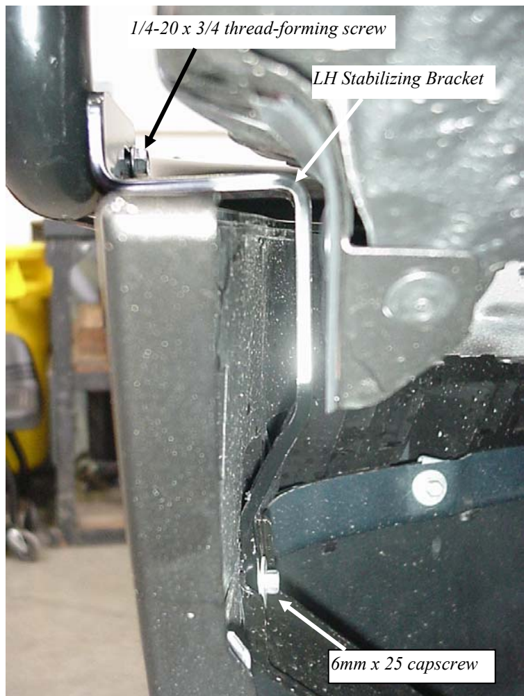
Figure 4 View inside left fender showing the Stabilizing Bracket installed
