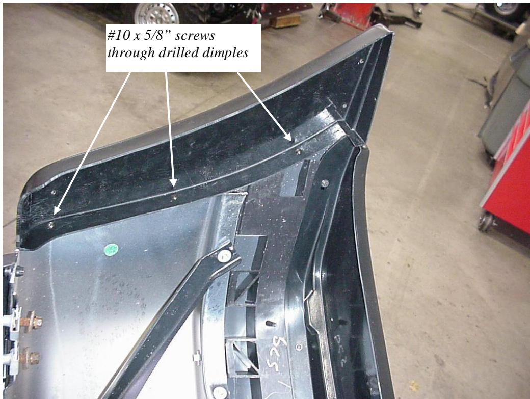
Figure 4 LH Endcap installed
