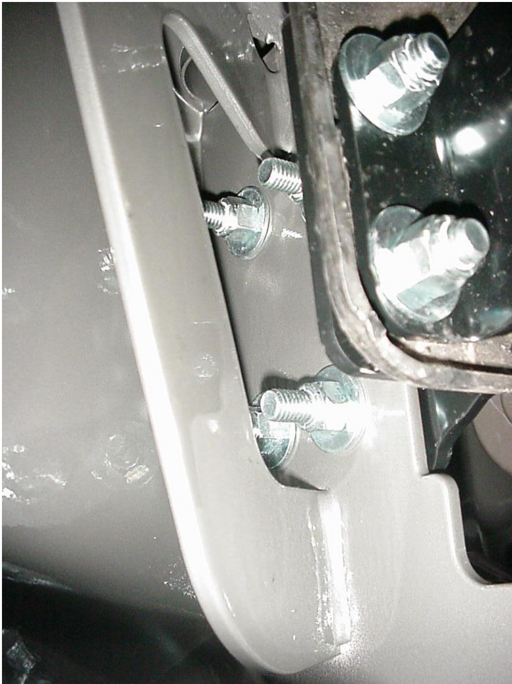
Figure 13: Tightening of bumper bolts. Driver's side shown.
