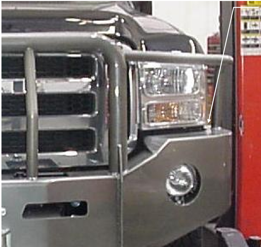
Figure 11: Shim adjustment and bumper to body clearance.
