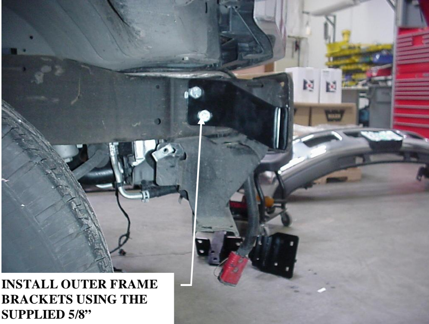
Figure 2: installation of outer frame bracket.
