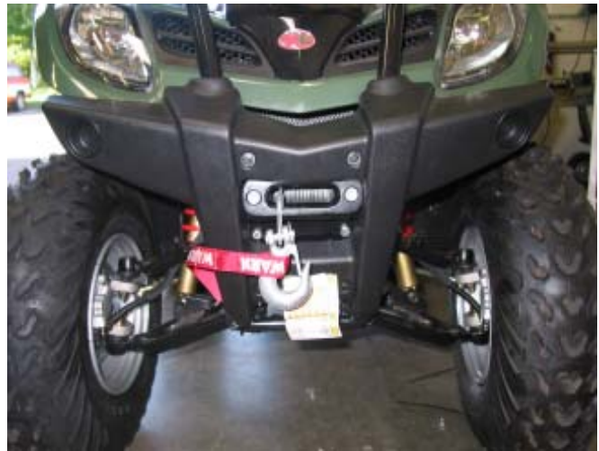
Figure 18: Completed Winch Installation on the Kymco MXU 250
