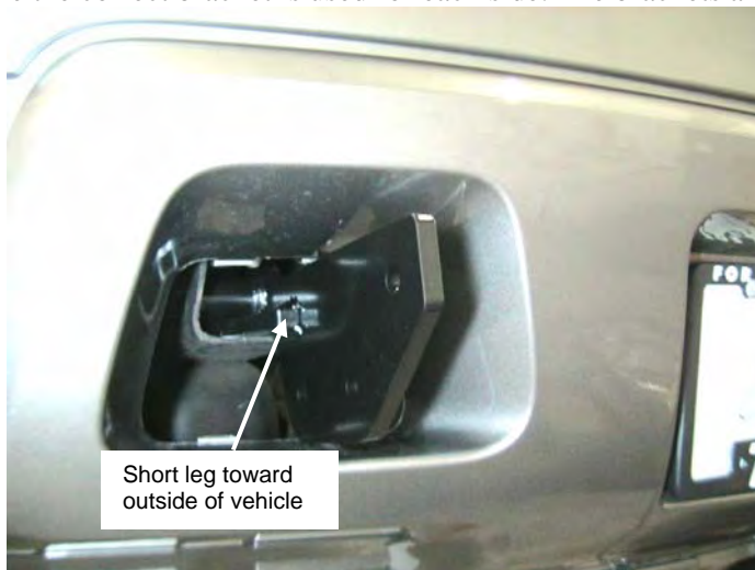
Figure 3 Frame Extension Installed
