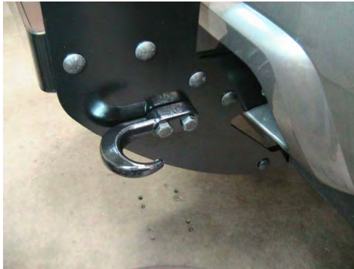
Figure 6 Installing Tow Hooks
