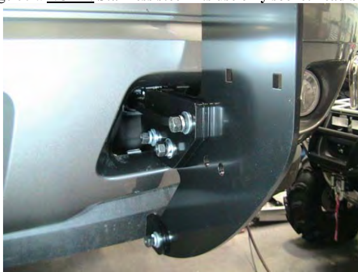
Figure 5. Mounting Side Member.
