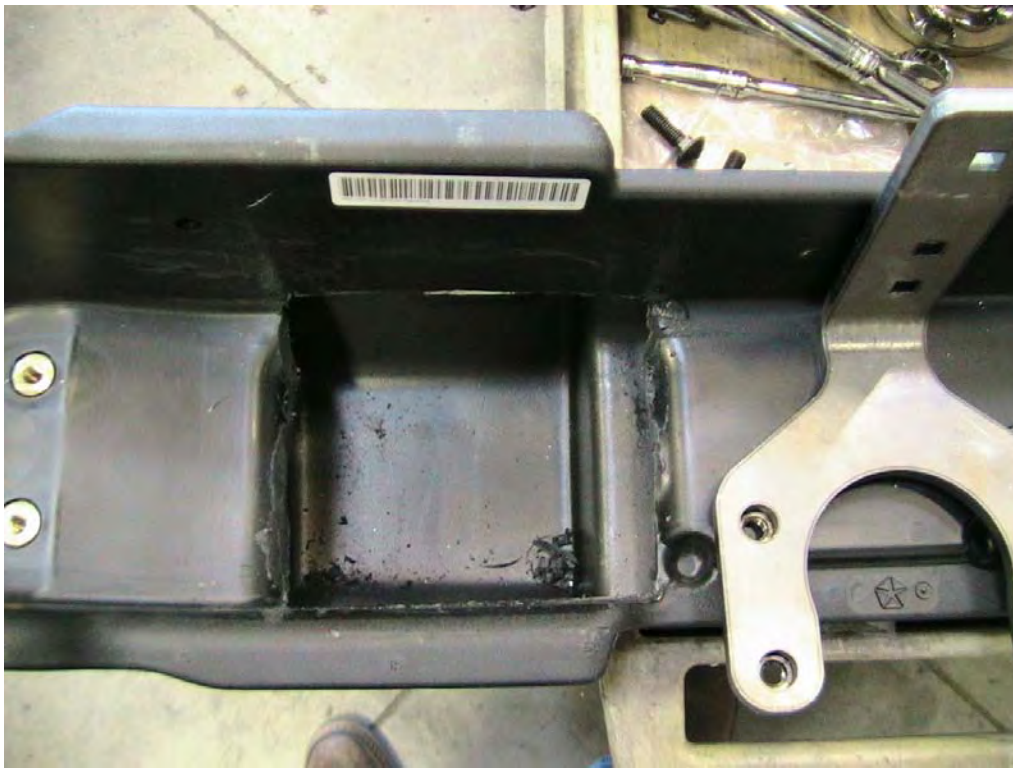
Figure 7: Cutout of inside of plastic bumper
