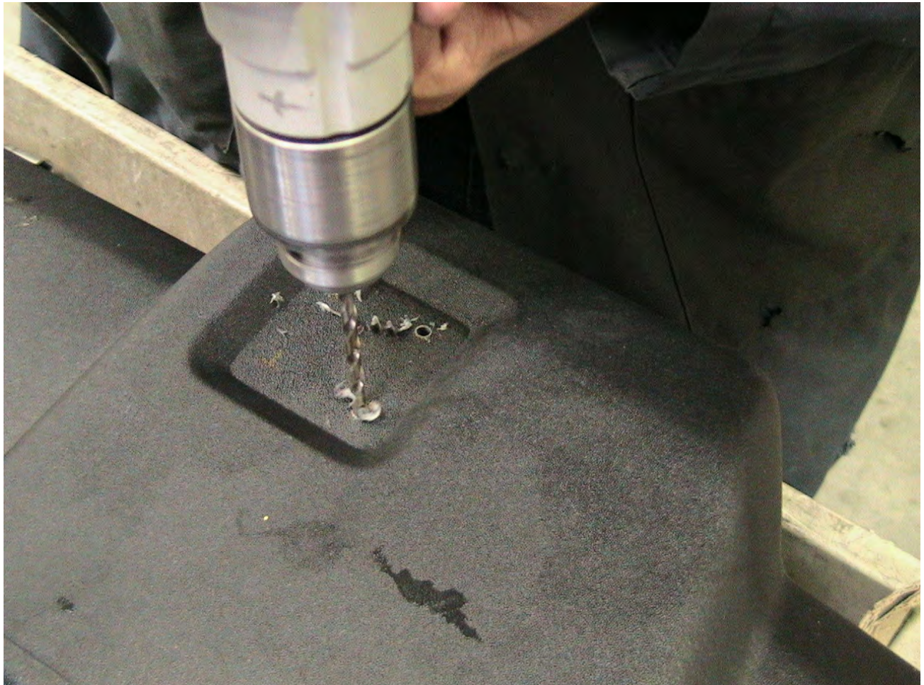
Figure 3: Drill corners of tow hook cutout
