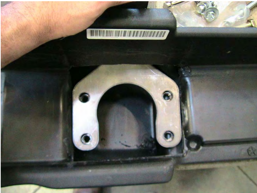
Figure 5: Tow hook fitment into plastic bumper
