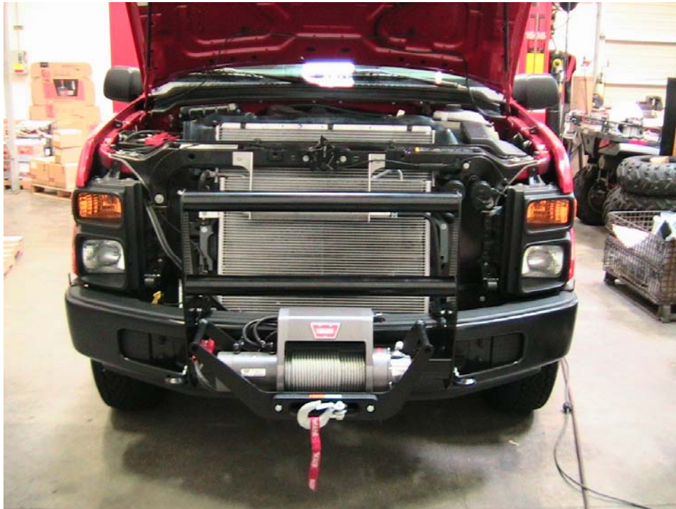
Figure 7. Finished kit (Multi-Mount winch shown.)
