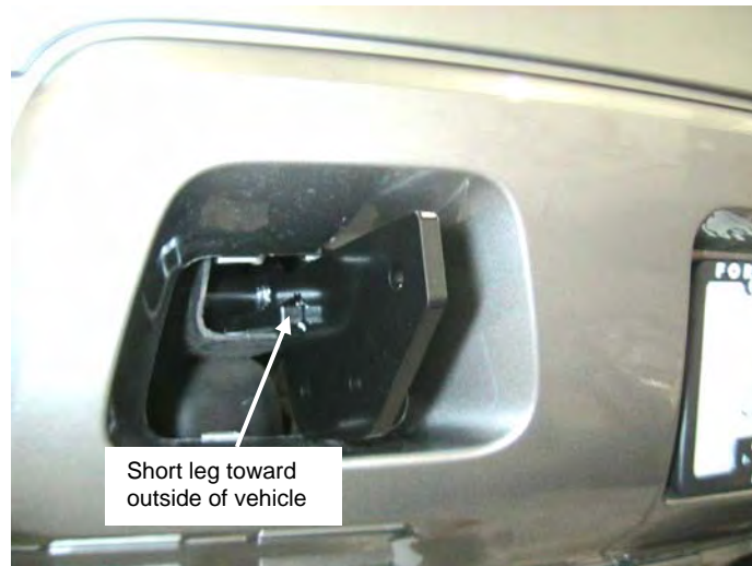
Figure 1 Frame Extension Installed (Tahoe shown - Suburban is similar)
