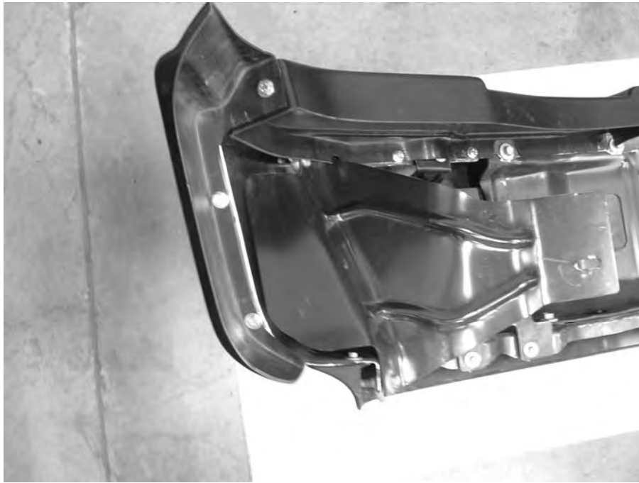
Figure 11 LH End Cap and Skirt installed
