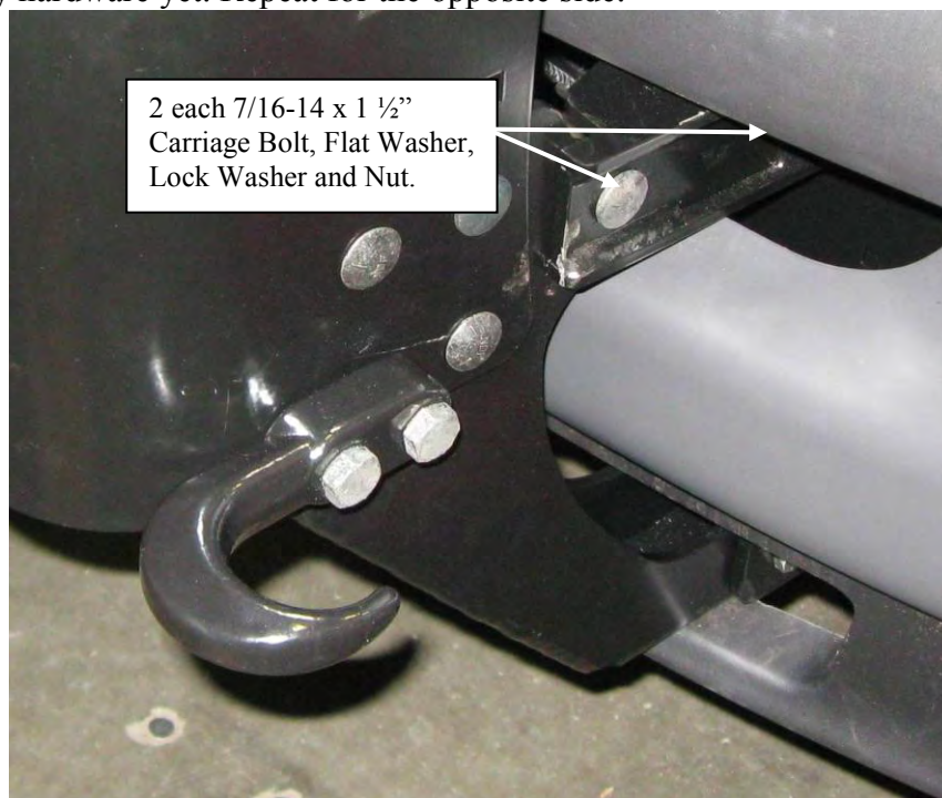
Figure 6: Large Frame Carrier: Top Carriage Bolt Positions.
