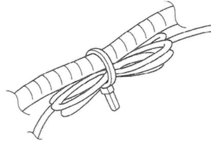
4. Use wire ties to securely attach wires to vehicle and bundle excess harness wires.
