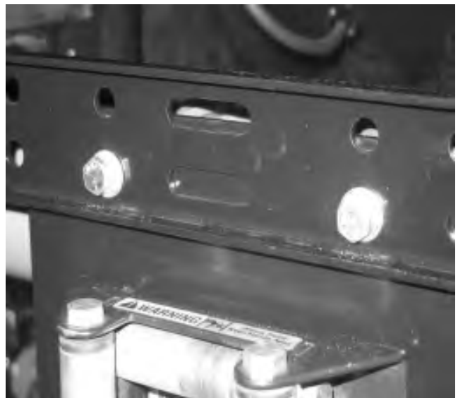
Figure 5, Attach winch and mounting plate
