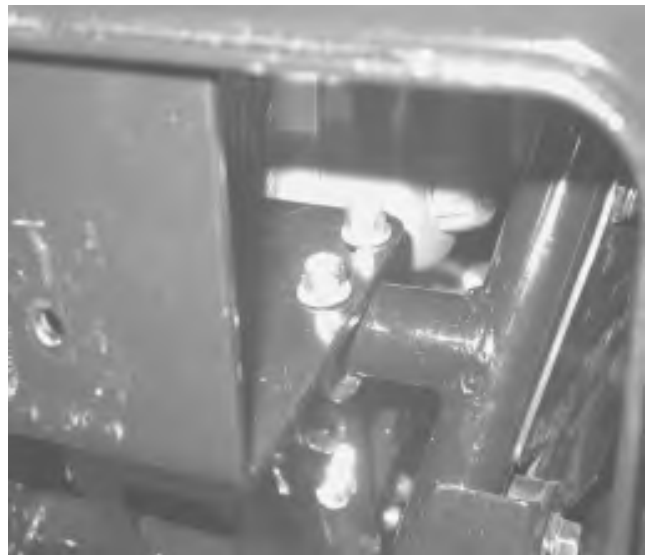
Figure 4, Fasten rear of mounting plate
