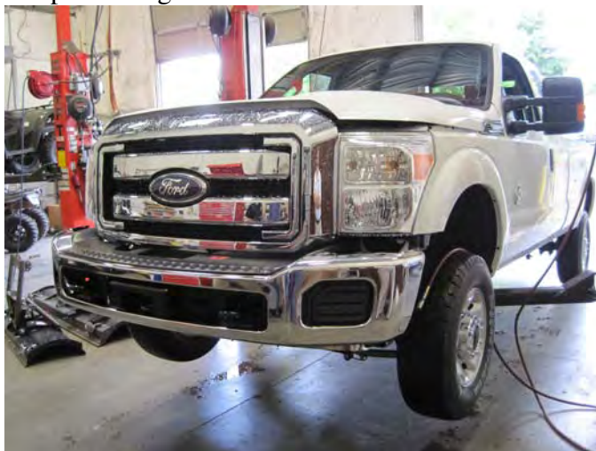
Figure 13: Bumper installed and leveled.
