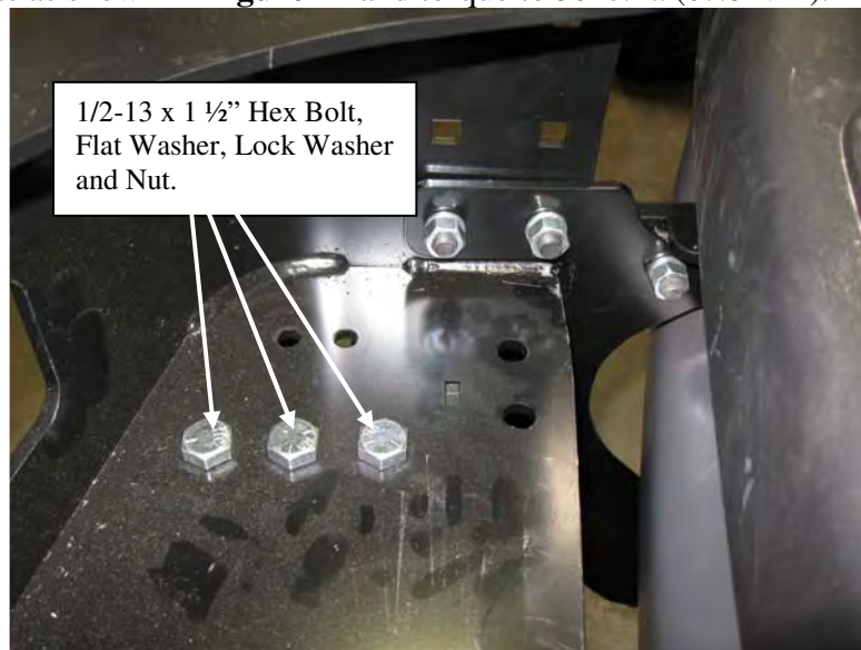
Figure 12: Large Frame Carrier: Carriage Hex Bolt Positions.
