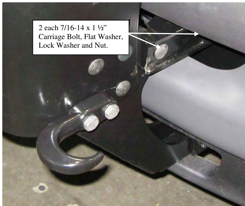
Figure 6: Large Frame Carrier: Top Carriage Bolt Positions.
