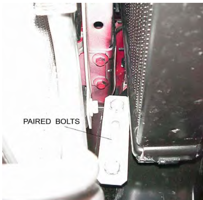
Figure BB: Bolts attaching bumper brackets to frame (viewed from center of vehicle, looking outward)
