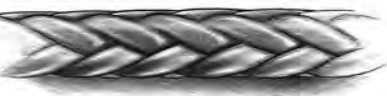
Rope exhibits fiber-set from compression. A slight sheen is visible. This is not a permanent characteristic and can be eliminated by flexing the rope.
