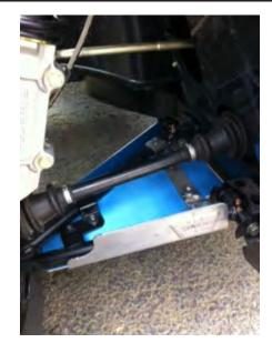
3. Attach the front right a-arm guard (A1) using 1 of the front brackets (B1) and 1 of the rear brackets (B2). Each bracket will be attached using the M8 flat hex head bolt, locking M8 hex nut and flat washer, see figure 2 and 3. Do not tighten all the fasteners down at this point, it will be easier to remove the protective covering before all the fasteners are torqued down.
