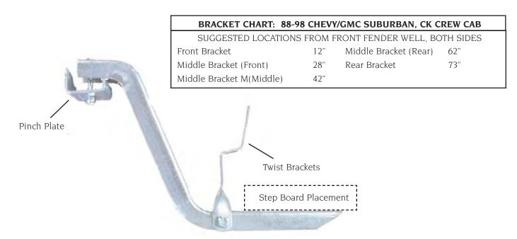
**STEP 3:** Attach the pinch plate portion of the brackets to the truck at the cab rail and tighten the 5/16" x 2½" Hex Head Bolts and 5/16" Nylocks. Note: All the brackets should be loosely hanging from the truck.
