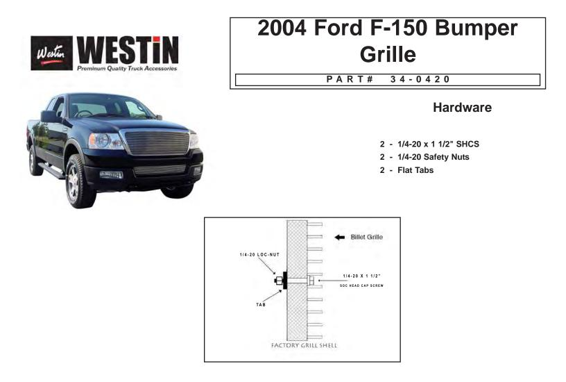
STEP 1 Center billet grille in lower bumper opening. Place 1/4-20 x 1 1/2" SHCS thru both Billet Grille & Factory Grille. Then place the supplied tabs & nuts on backside of facory grille as shown above and tighten.
