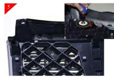
Using a cut off wheel or hack saw. Cut off 1/4" of the bolts located along the top outer sections only. You do not need to cut off the remaing bolts. Next replace the plastic covers that were removed in step 3.
