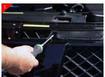
Remove the stock grille shell by using a straight blade screw driver and turing the Plastic Hold Downs a quarter turn to release. There are (4) across the top and (3) on the bottom and (4) on the left and right side. Step 2 will show the locations of the left and right release screws that are not visible in the lower corners of the stock grille.
