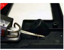
B: Using a saw, remove the (2) raised bosses on the back of the holder.
