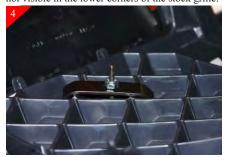
Insert the billet grille and center into the openings. Use the supplied hardware to attach the billet grille to the factory grille shell. Tighten all bolts, being careful not to over tighten. As shown above.
