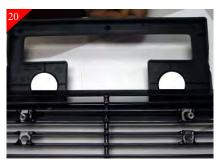
C: Attach the holder using the supplied #10 x 2" bolts and nuts thru the bottom most tabs on the billet grille.
