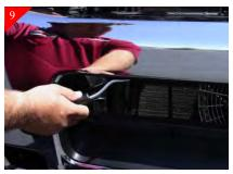
Next remove the (3) Plastic Push Rivets located along the top. Then remove the plactic insert.
