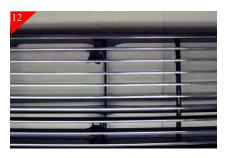
Center the Billet grille in the plastic shroud with the polished surface flush with the face of the shroud as shown.
