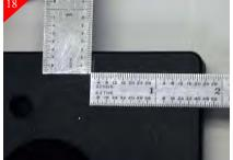
A: At each corner drill a 3/16" hole 1 3/4" from the outside top edges and 3/8" down from the top edges as shown above.
