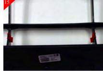
Place the U-Clips over the (4) holes just drilled as shown. Only the bottom 2 are shown above.
