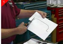
(Fig B) shown above is the template to be used for the rest of the trimming process of the shell. The full scale template to be used is on the following page. You will need to cut out template as shown. Keep top portion.
