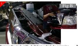
Remove the stock grille shell from vehicle by removing the 2 bolts along the top of the grille shell and then the bottom of the grille shell is held by 2 snap clips. With the top 2 bolts removed lean the grille shell forward and reach behind and release (Fig. B)
