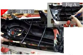
Next you will be removing the center section of the stock grille. Using a hack saw blade or cut off wheel remove as shown above (Fig A). Making sure to leave material for finish sanding. (Fig B) showing center section removed.
