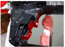
After removing the center section you will need to trim the access material away from the drivers & passengers side of the grille shell shown above in RED.
