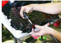
Then attach billet grille using the supplied #8 x 5/8" phil pan head screw and U-Clips as shown above. Take note that the U-Clip goes on the outside of the grille shell shown above in RED. Tighten all hardware. Then re-install grille back on vehicle.
