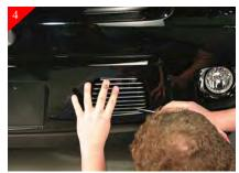
Place billet grille into opening and center. Then using a 90° scribe mark the location of the holes in bracket where it meets the vehicle.
