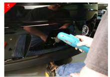
Remove the billet grille from opening and also remove the brackets from the billet grille. Then drill a 3/16" hole in each of the just marked locations.
