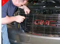
Simply tighten up the toggle bolts. To help start bolts it maybe necessary to pull out on the billet grille so that there is something for the bolt to tighten against. Another method is to use a second screwdriver to help hold the wing nut until it snugs up against the shell.
