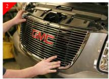
Place billet grille into opening and center. Then push the toggle bolts thru as shown above.
