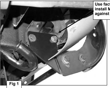
Use factory hex bolts to install Mounting Brackets against frame channel
