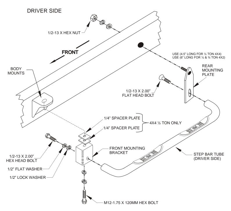
ASSEMBLY AND INSTALLATION VIEW OF DRIVER SIDE - PASSENGER SIDE OPPOSITE
