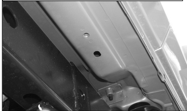
(Fig 2) Example of 2010-12 "closed" floor panel with threaded hole-Nut Plate not required
