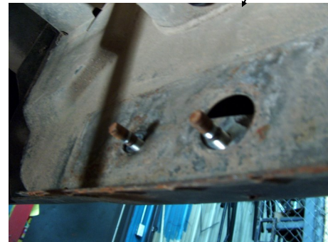
1997-98 EXTENDED CAB 3 DOOR DRIVER SIDE REAR ONLY. BOLT PLATE INSTALLATION FIGURE 4
