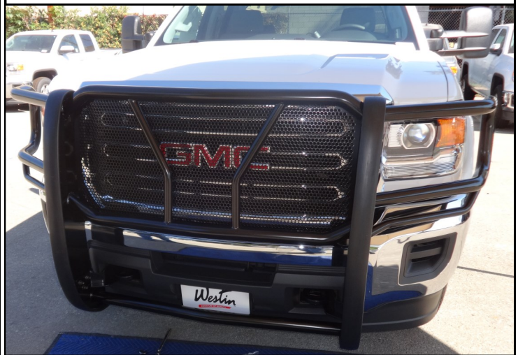
HDX GRILLE GUARD, INSTALLATION COMPLETE
